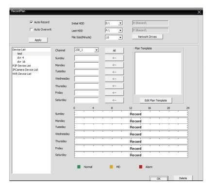
After checking the automatic video, according to user requirements you can configure the video plan. Select respectively, recorded on path, whether you need to loop video, video package length (time), the video time setting, and video channels. The following chart:
